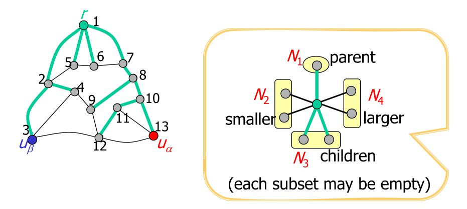
(ost1) For each edge not in the tree *T*, none of the endpoints is an ancestor of the other in *T*.
