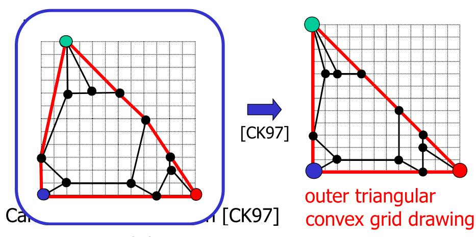
convex grid drawing but not outer triangular convex grid drawing
