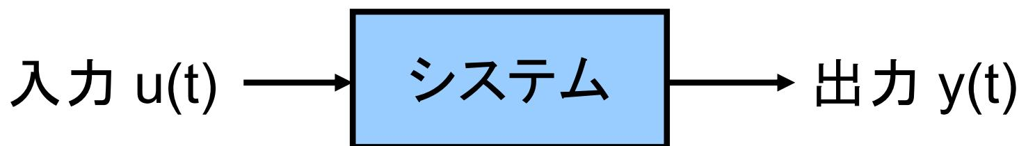
$$\begin{aligned} & a_n \frac{d^n y(t)}{dt^n} + a_{n-1} \frac{d^{n-1} y(t)}{dt^{n-1}} + \cdots + a_0 y(t) \\ & = b_m \frac{d^m u(t)}{dt^m} + b_{m-1} \frac{d^{m-1} u(t)}{dt^{m-1}} + \cdots + b_0 u(t) \end{aligned}$$
