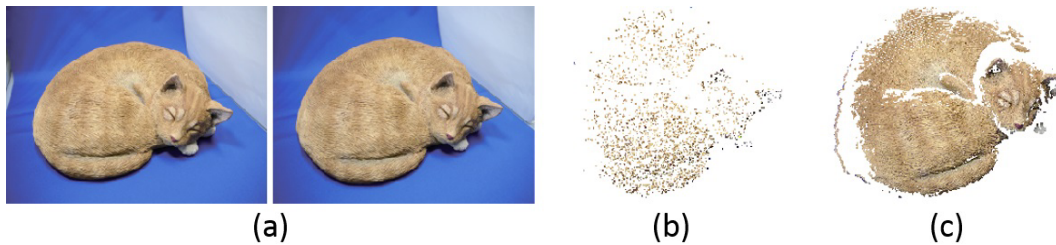
Fig. 8: Results of 3D measurement: (a) input stereo image pair, (b) 3D points measured by SIFT-based SfM (2790 points) and (c) 3D points measured by the proposed procedure (25 243 points).
