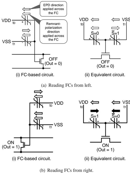
FIGURE 7 Relationship between the reading path and the output *Out*.
