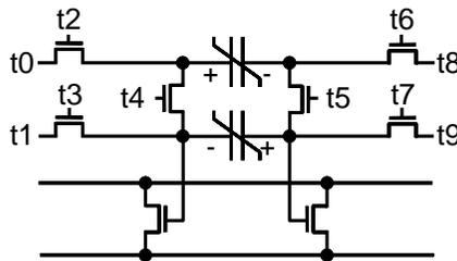
FIGURE 8 Structure of the FFC element.
