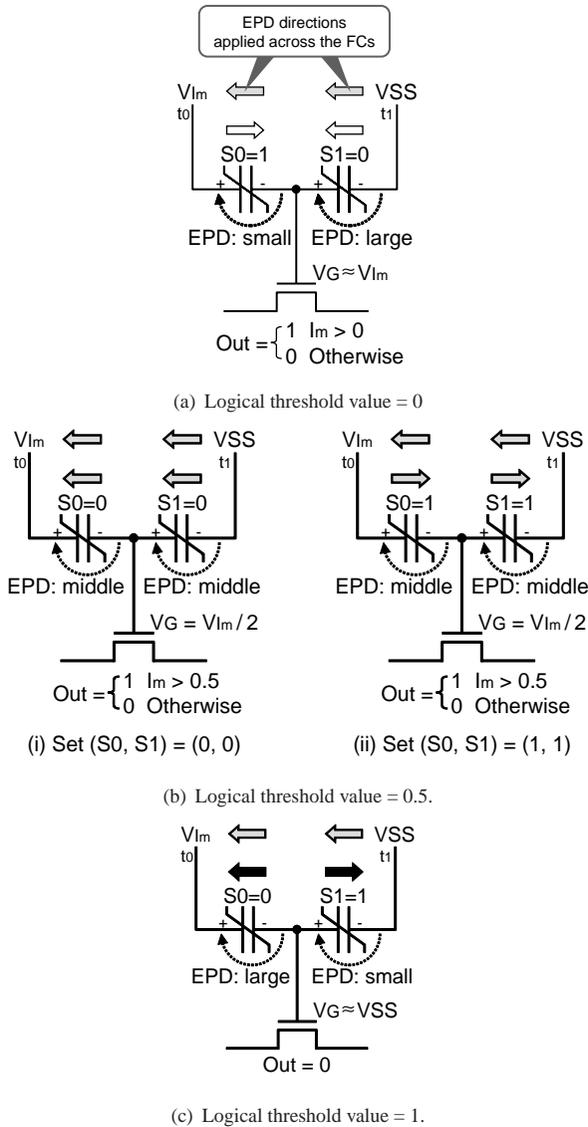
FIGURE 19 Fundamental principle of a multiple-valued FFC element.
