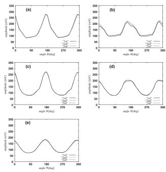
Fig. 3. Maximum amplitude of the received signals at each azimuth angle  $\theta$ . (a)  $\phi_1 = \phi_2 = 30^{\circ}$ . (b)  $\phi_1 = \phi_2 = 40^{\circ}$ . (c)  $\phi_1 = \phi_2 = 50^{\circ}$ . (d)  $\phi_1 = \phi_2 = 60^{\circ}$ . (e)  $\phi_1 = \phi_2 = 70^{\circ}$ .
