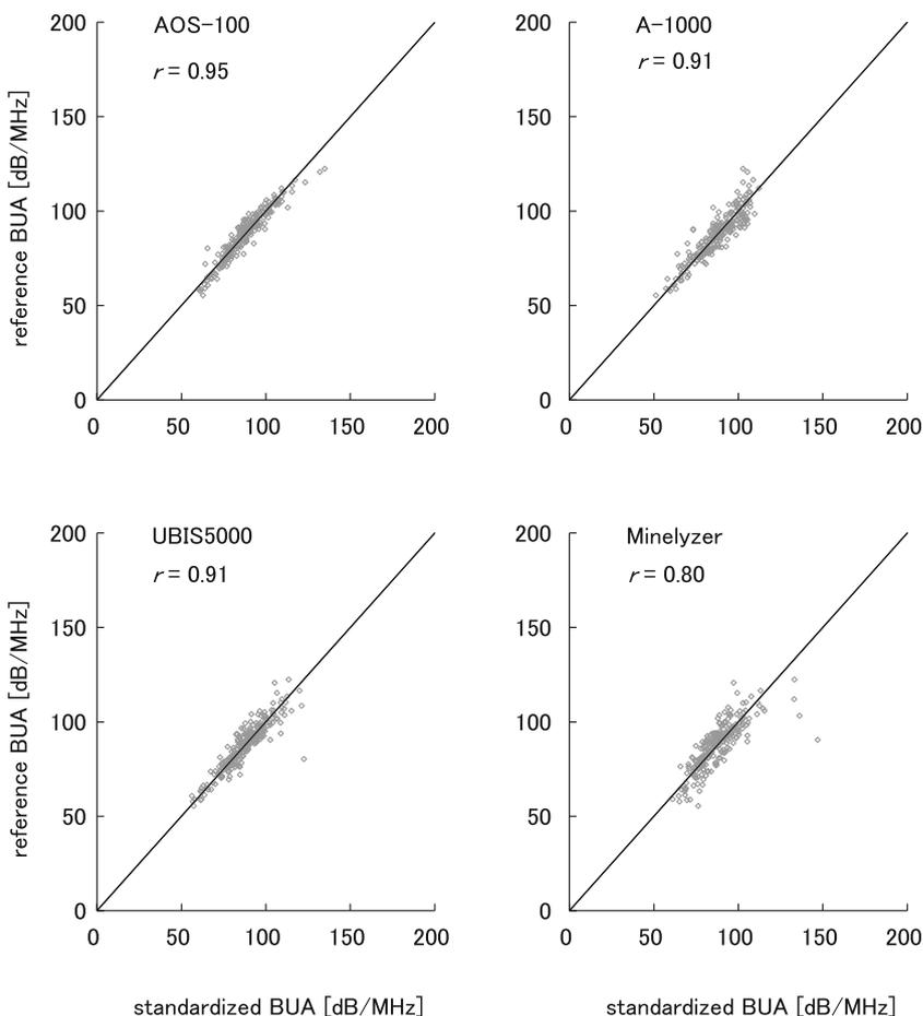
**Fig. 10** Subject measurement results for standardized BUA. The mean BUA (reference BUA) has been arranged in ascending order from lowest to highest, and the standardized BUA for each model is also shown
