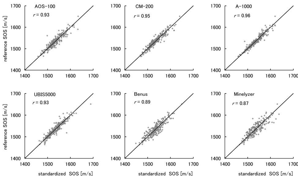
**Fig. 6** Subject measurement results for standardized SOS. The mean SOS (reference SOS) has been arranged in ascending order from lowest to highest, and the standardized SOS for each model is also shown
