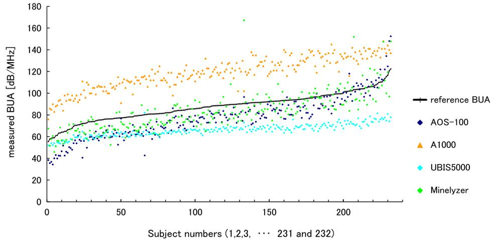
**Fig. 8** Results of regression analysis of the reference BUA and the measured BUA values for each model ( $p < 0.0001$ ) (regression analysis: standard major axis regression analysis)
