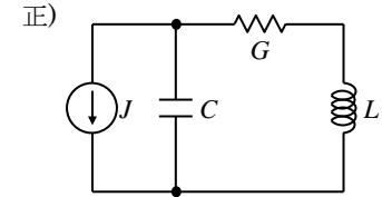
$$\text{正)} \quad [F_\pi] = \begin{bmatrix} 1 & 0 \\ \frac{1}{Z_{31}} & 1 \end{bmatrix} \begin{bmatrix} 1 & Z_{12} \\ 0 & 1 \end{bmatrix} \begin{bmatrix} \frac{1}{Z_{23}} & 0 \\ 1 & 1 \end{bmatrix} = \begin{bmatrix} 1 + \frac{Z_{12}}{Z_{23}} & Z_{12} \\ \frac{1}{Z_{31}} + \frac{Z_{12}}{Z_{23}Z_{31}} + \frac{1}{Z_{23}} & 1 + \frac{Z_{12}}{Z_{31}} \end{bmatrix} \quad (6.53)$$
