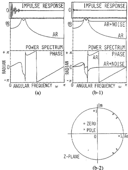
Fig. 3. The characteristics of the AR model (for the first example). (a) The fourth-order AR model of (31). (b-1) AR model buried in the white noise (SNR = -5 dB). (b-2) The poles of the AR model and the spectral zeros introduced by the additive noise.
