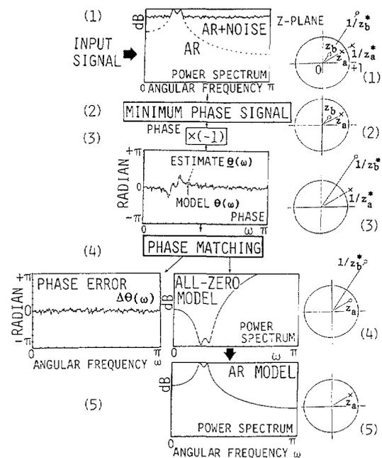
Fig. 1. Illustration showing the procedure of the proposed method for estimation of the parameters of the AR process in white noise.
