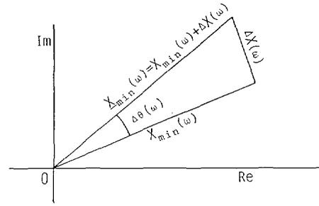
Fig. 2. Illustration showing the phase error  $\Delta\Theta(\omega)$  in the minimum phase model  $X_{\min}(\omega)$  which is reconstructed from the power spectrum of the observed signal  $y(n)$ .
