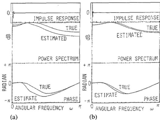
Fig. 8. The estimated power spectrum and phase obtained by the two methods (for the second example (SNR = +4 dB)). (a) OMYW method. (b) The proposed method.
