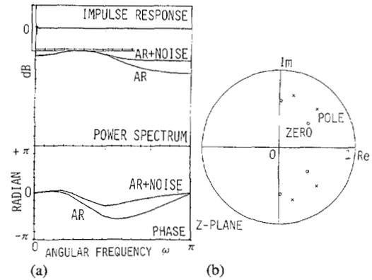
Fig. 7. The characteristics of the AR model (for the second example). (a) The fourth-order AR model of (33) and the AR model buried in the white noise (SNR = +4 dB). (b) The poles of the AR model and the spectral zeros introduced due to the additive noise.
