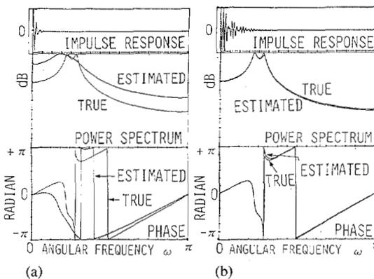
Fig. 6. The estimated power spectrum and phase obtained by the two methods (for the first example) (SNR = -5 dB). (a) OMYW method. (b) The proposed method.
