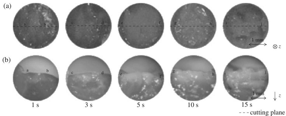
Fig. 6. Results of the cutting test using the 60-kHz knife. (a) Tissue surface after the cutting test. (b) Cross-sectional views along broken lines in (a).
