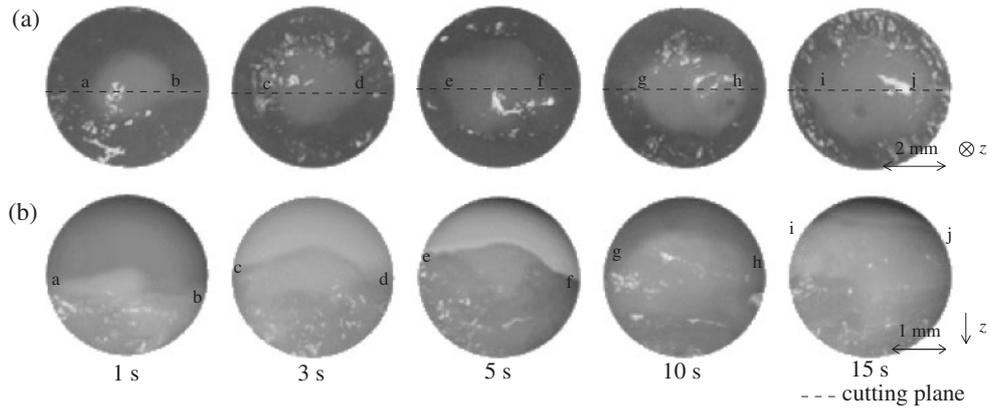
Fig. 4. Results of the cutting test using the 20 kHz knife. (a) Tissue surface after the cutting test. (b) Magnified cross-sectional views along broken lines in (a).
