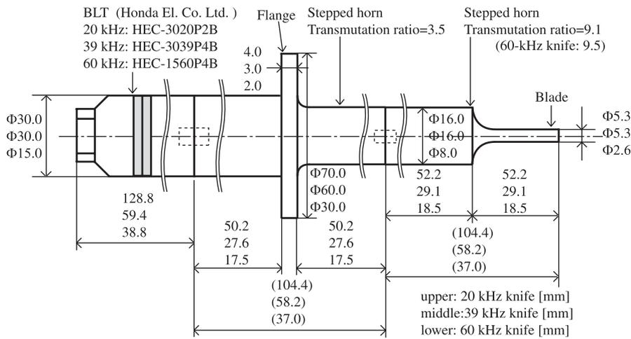
Fig. 1. Technical drawing of the prototype knife.
