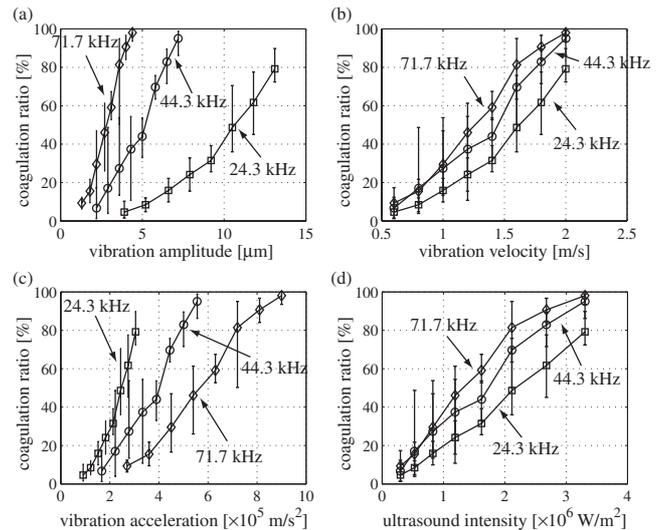
Fig. 8. Measured coagulation ratio versus (a) vibration amplitude, (b) vibration velocity, (c) vibration acceleration, and (d) ultrasound intensity.
