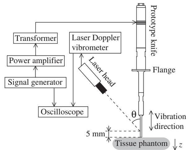
Fig. 3. Experimental setup for measurement of frequency characteristic.
