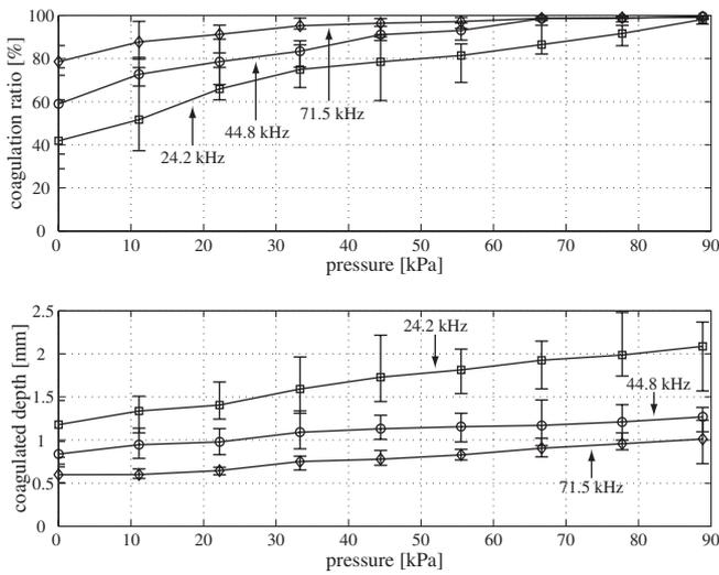
Fig. 14. Relationship between load and tissue coagulation. (a) Coagulation ratio. (b) Coagulated depth.
