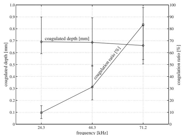
Fig. 10. Results of measuring the coagulation ratio and the coagulated depth at a constant vibration amplitude (4  $\mu$ m) for each operation frequency.
