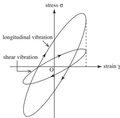
Fig. 21. Illustration of stress–strain diagrams for different vibration modes.
