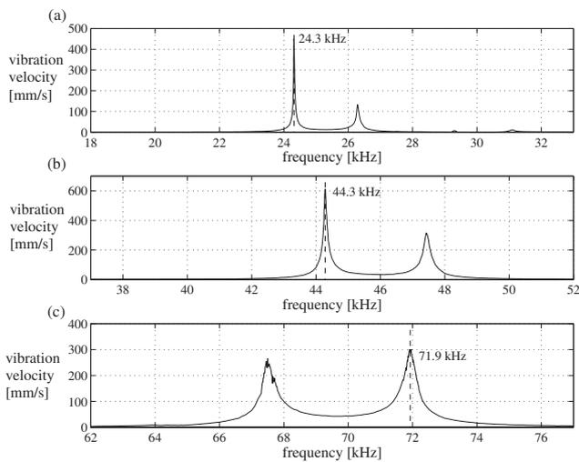
Fig. 2. Frequency response of vibration velocity of the tip of the knife.
