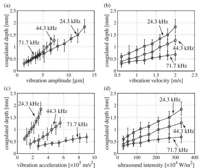
Fig. 9. Measured coagulated depth versus (a) vibration amplitude, (b) vibration velocity, (c) vibration acceleration, and (d) ultrasound intensity.
