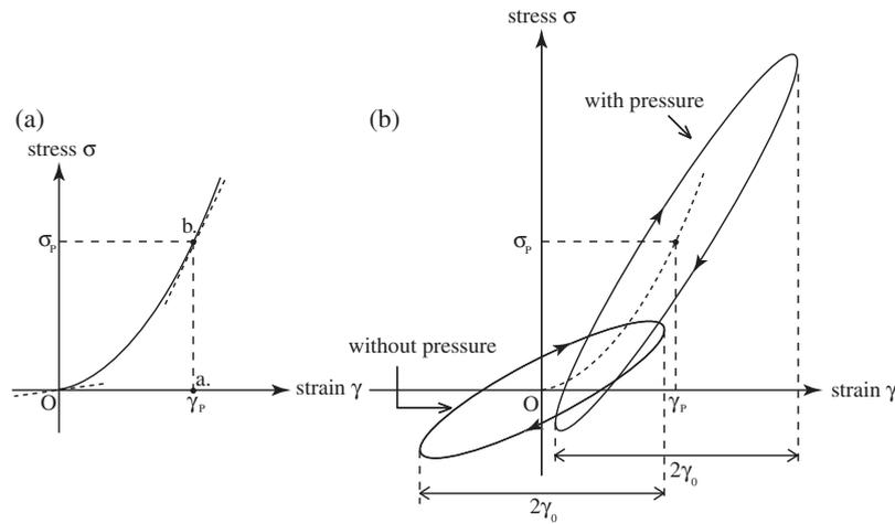
Fig. 20. Illustrations of (a) change in elasticity due to the static pressure and (b) change in hysteresis property due to static pressure.
