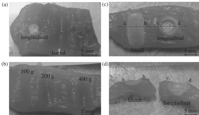
Fig. 16. Difference in tissue coagulation depending on (a) vibration direction (vibration velocity = 2 m/s, load = 200 g, driving period = 10 s), (b) pressure load (lateral vibration, vibration velocity = 2 m/s, driving period = 20 s, tissue load = 100 g (left), 200 g (center), and 400 g (right)), and (c) vibration direction (vibration velocity = 4 m/s, load = 200 g, driving period = 10 s). (d) Cross-sectional view of (c).
