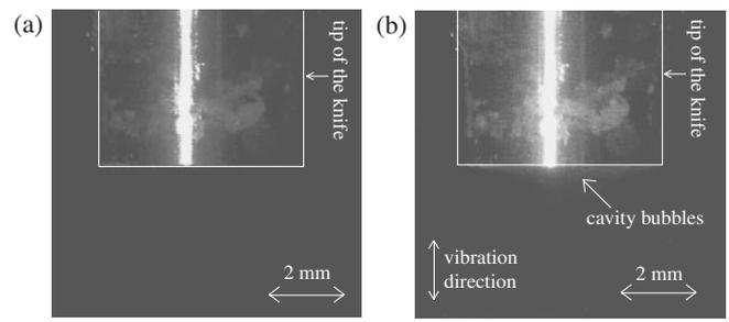
Fig. 13. Magnified view of the tip of the knife. (a) Before operation. (b) During operation.
