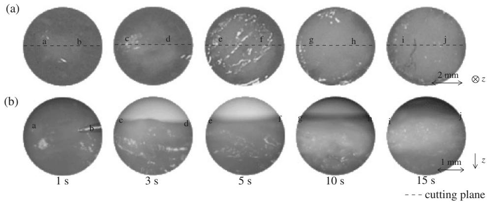
Fig. 5. Results of the cutting test using the 40-kHz knife. (a) Tissue surface after the cutting test. (b) Magnified cross-sectional views along broken lines in (a).
