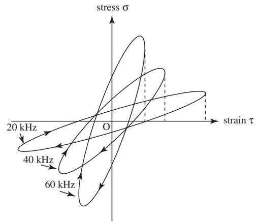
Fig. 19. Stress–strain diagrams at different frequencies.
