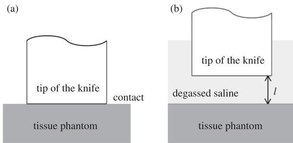
Fig. 11. Experimental setup. (a) Tip of the knife was kept contact with the surface. (b) Tip of the knife was separated from the tissue surface.
