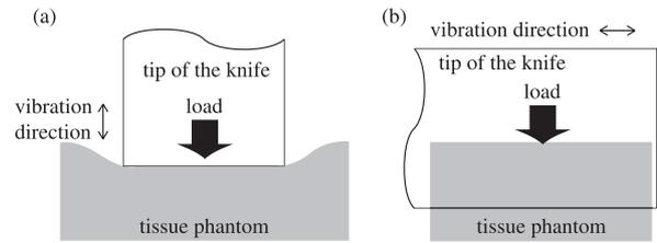
Fig. 15. Experimental setup for investigating the tissue coagulation depending on vibration direction. (a) Longitudinal direction. (b) Lateral direction.
