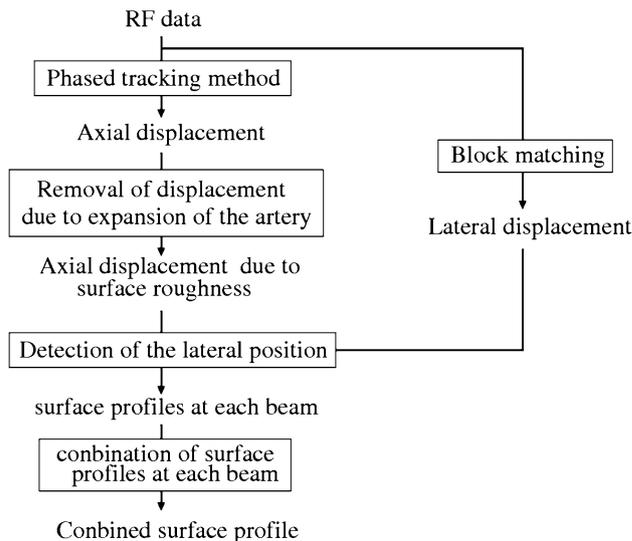
Fig. 2 Procedure for measurement of surface roughness
