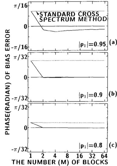
Fig. 10. Relation between the number  $M$  of blocks used in the proposed method and the phase of the bias error  $\Delta\widehat{H}_{bk}(k)$  in (33) near the resonant frequency  $k_1 = 10$  under the condition that the total signal length  $MN$  is always equal to 64.  $Lp_1 = \frac{2\pi}{7}$ . The dotted line shows the bias error in the estimate  $\widehat{H}_{all}(k)$  of the standard cross spectrum method: (a)  $|p_1| = 0.95$ ; (b)  $|p_1| = 0.9$ ; (c)  $|p_1| = 0.8$ .
