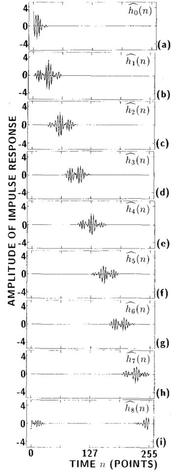
Fig. 12. Impulse response estimates  $\widehat{h}_i(n)$ , ( $i = 0, 1, \dots, 8$ ), which are obtained by applying DFT to the block transfer function estimates  $\widehat{H}_i(k)$  multiplied by shift coefficients  $\exp(-j2\pi \cdot ki/M)$ . In the proposed method in Section III, each segment with length  $MN = 128$  is divided into nonoverlapping 8 blocks, where each has 32 points in length ( $M = 8$ ,  $N = 32$ ).
