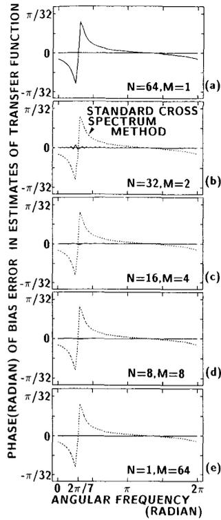
Fig. 8. Phase characteristics of the bias error in the estimate  $\widehat{H}_{bk}(k)$  by the proposed method in (32) for different five combinations of the number  $M$  of the blocks and the length  $N$  of a block. The dotted line shows the bias error  $\Delta\widehat{H}_{all}(k)$  in the estimate  $\widehat{H}_{all}(k)$  of the standard cross spectrum method in (30): (a)  $N = 64, M = 1$ ; (b)  $N = 32, M = 2$ ; (c)  $N = 16, M = 4$ ; (d)  $N = 8, M = 8$ ; (e)  $N = 1, M = 64$ .
