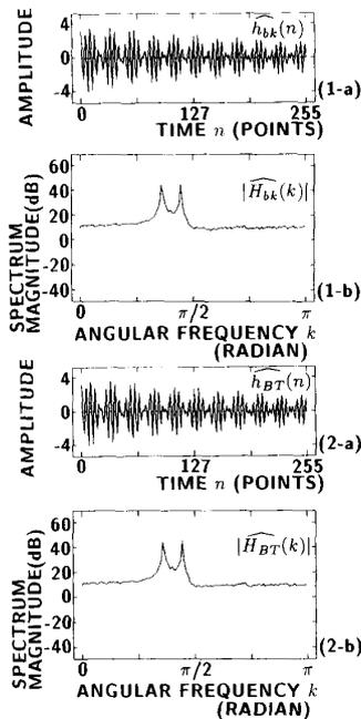
Fig. 14. (1) Transfer function estimate  $\widehat{H}_{bk}(k)$  and its impulse response  $\widehat{h}_{bk}(n)$  obtained by the proposed method described in Section III ( $M = 8$ ,  $N = 32$ ); (2) transfer function estimate  $\widehat{H}_{BT}(k)$  and its impulse response  $\widehat{h}_{BT}(n)$  obtained by the proposed method described in Section IV-D ( $M = 128$ ,  $N = 1$ ).
