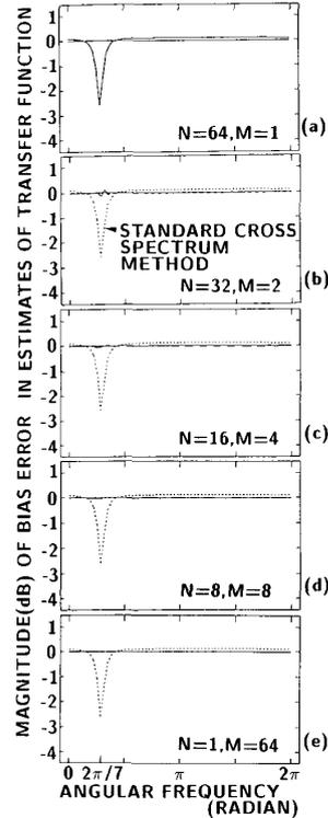
Fig. 7. Magnitude characteristics of the bias error in the estimate  $\widehat{H}_{bk}(k)$  by the proposed method in (32) for different five combinations of the number  $M$  of the blocks and the length  $N$  of a block. The dotted line shows the bias error  $\Delta \widehat{H}_{all}(k)$  in the estimate  $\widehat{H}_{all}(k)$  of the standard cross spectrum method in (30): (a)  $N = 64, M = 1$ ; (b)  $N = 32, M = 2$ ; (c)  $N = 16, M = 4$ ; (d)  $N = 8, M = 8$ ; (e)  $N = 1, M = 64$ .
