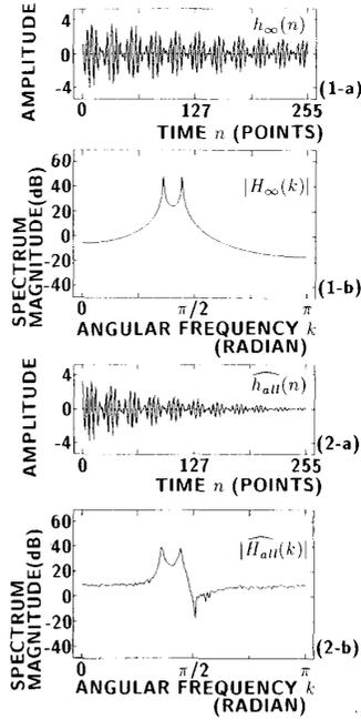
Fig. 11. (1) Magnitude characteristics of the fourth-order all-pole transfer model  $H_\infty(k)$  employed in the computer simulation in Section VI and its impulse response  $h_\infty(n)$ ; (2) transfer function estimate  $\widehat{H}_{\text{all}}(k)$  and its impulse response  $\widehat{h}_{\text{all}}(n)$  obtained by the standard method described in Section II.
