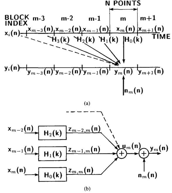
Fig. 3. When the impulse response is long, the signal transmission system model of single input/single output in Figs.1 and 3(a) is also described by the multiple input/single output transfer system as shown in Fig. 3(b).
