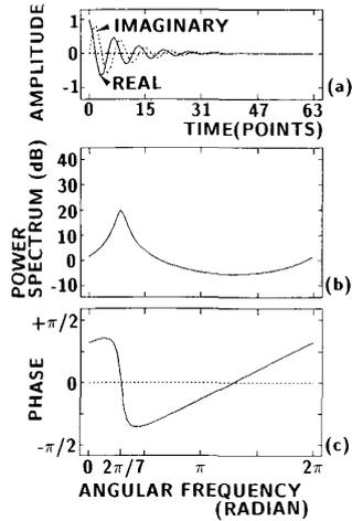
Fig. 6. (a) Examples of the impulse response  $h(n)$  in (15) employed in Figs. 7 and 8; (b), (c) frequency characteristics  $H_{\infty}(k)$  of the signal in Fig. 6(a) defined by (18). The order  $P$  of the rational transfer function is equal to 1,  $C_1 = 1$ ,  $|p_1| = 0.90$ , and  $\angle p_1 = \frac{2\pi}{7}$ . The length  $MN$  is equal to 64.
