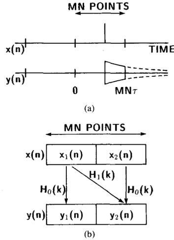
Fig. 2. (a) Impulse response is dropped at the end of the block in the standard method. (b) Illustration explaining the cause of the bias error in the estimates obtained by the standard method.
