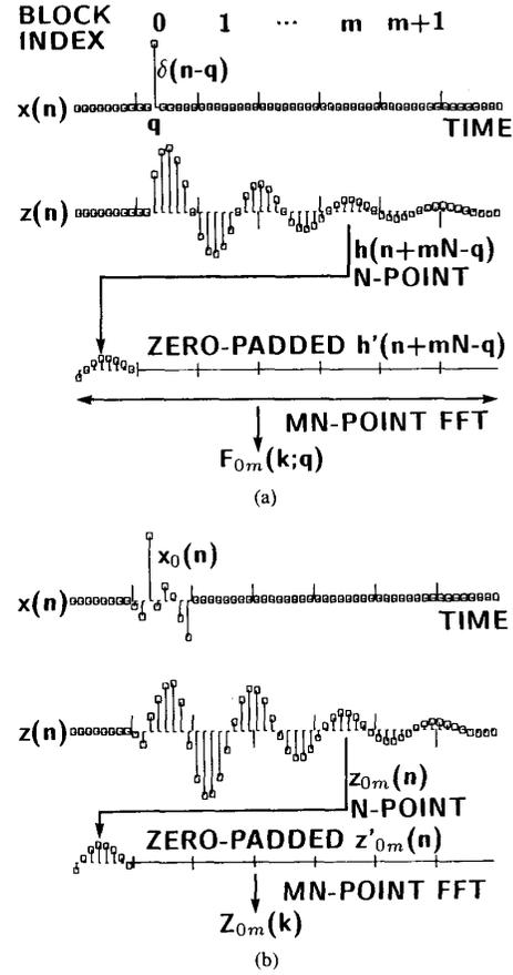
Fig. 4. (a)  $F_{0m}(k; q)$  denotes the  $MN$ -point spectrum of the zero-padded signal  $h'(n + mN - q)$  in the  $m$ th block of the response of the transfer system to the impulse  $\delta(n - q)$  at a time  $q$  in the 0th block; (b)  $Z_{0m}(k)$  denotes the  $MN$ -point spectrum of the  $N$ -point signal  $z_{0m}(n)$  in the  $m$ th block of the response of the transfer system to the input signal  $x_0(n)$  in the 0th block.
