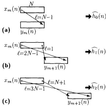
Fig. 13. Illustrations for explaining the relations between the length  $\ell$  of the estimated impulse response in Fig. 12 for each block transfer function and the amount of time for which the output block is delayed from the input block.
