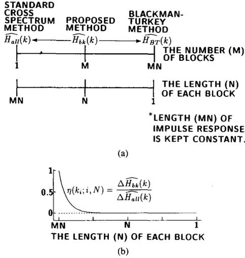
Fig. 5. (a) Relation among the proposed method, the standard cross spectrum method, and the Blackman-Tukey method; (b) theoretical ratio  $\eta(k; i, N)$  of  $\Delta\widehat{H}_{bk}(k)$  in (33) to  $\Delta\widehat{H}_{all}(k)$  in (31) is always equal to or less than 1 for various lengths  $N$  of each block.
