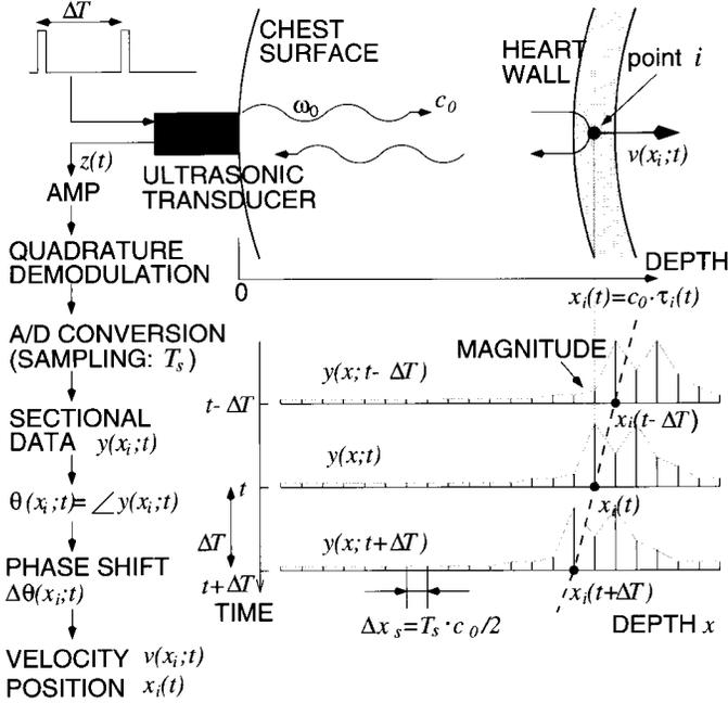
Fig. 2. Schematic representation of the principle of the transcutaneous detection of a velocity signal  $v(x_i, t)$  and the instantaneous position  $x_i(t)$  of the  $i$ th point in the heart wall using pulsed ultrasound from the chest wall.
