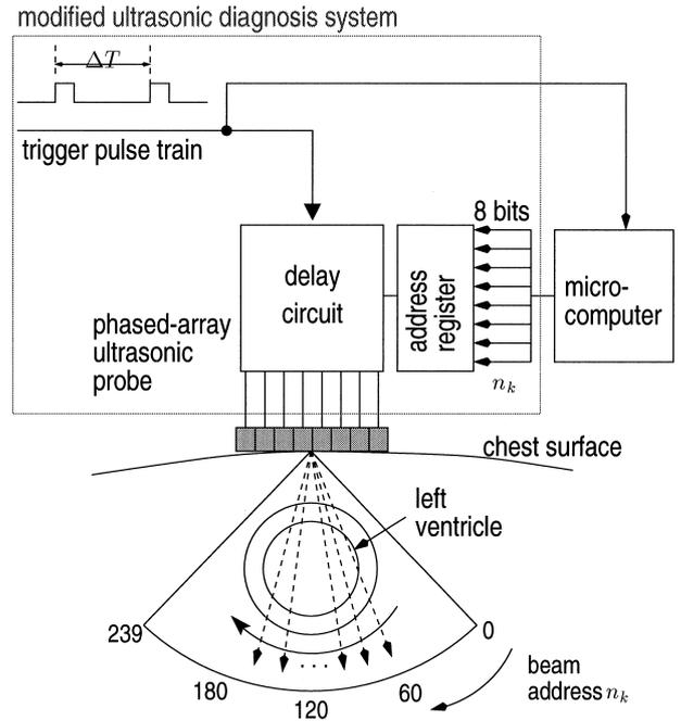
Fig. 3. A diagram illustrating simultaneous measurement of the velocity signals at multiple points on the LV wall by selecting 10 scan lines with directions  $\{\theta_k\}$  from a sector scanner in real-time using a microcomputer.
