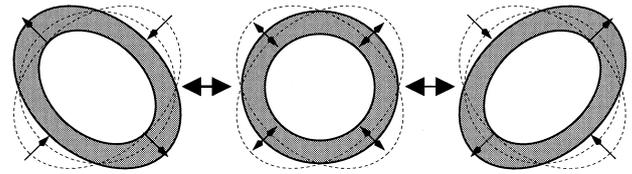
Fig. 2. Three phases of a mode-2 vibration of an elastic spherical shell.
