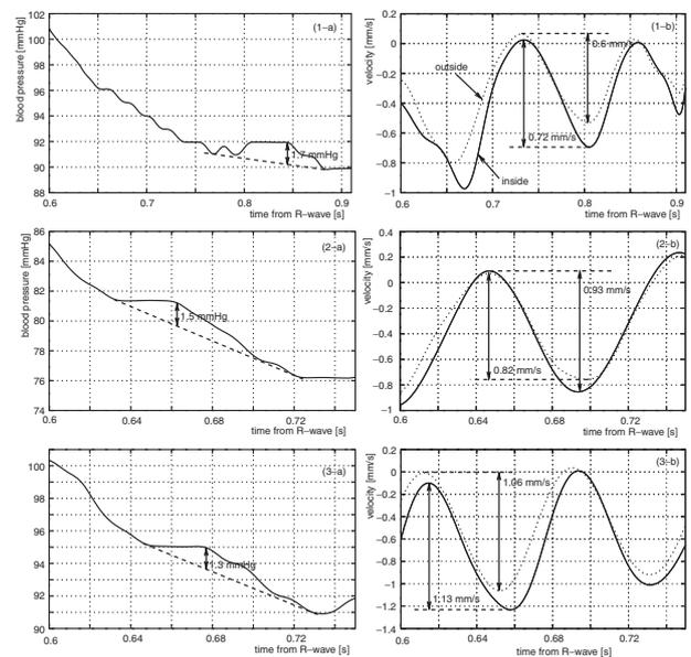
Fig. 12. Blood pressure and velocity after 0.6s from the R-wave of electrocardiogram. (1) 7.5 Hz. (2) 10 Hz. (3) 12.5 Hz. (a) Blood pressure. (b) Velocities at the intimal side and the adventitial side.
