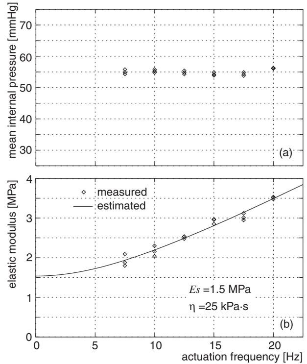
Fig. 8. (a) Mean internal pressure. (b) Elastic moduli,  $|E_{inc}^h(f_{ac})|$ , measured at each actuation frequency,  $f_{ac}$ , using the laser line gauge (plot), and the estimated Voigt model (solid curve).
