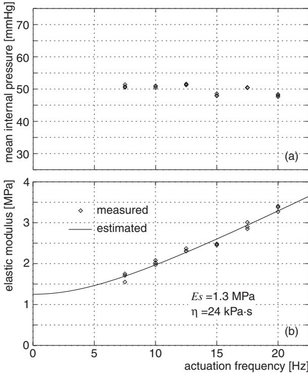
Fig. 7. (a) Mean internal pressure. (b) Elastic moduli,  $|E_{\theta}^h(f_{ac})|$ , measured at each actuation frequency,  $f_{ac}$ , using ultrasound (plot), and the estimated Voigt model (solid curve).
