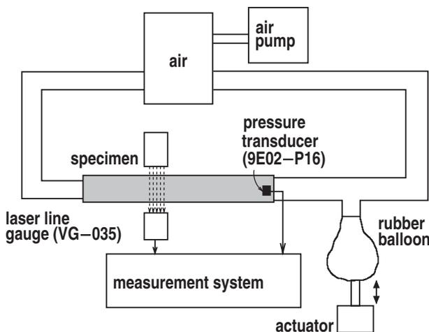
Fig. 4. Experimental system employed for testing the relationship between the internal pressure,  $\Delta p(t)$ , and the external diameter,  $2\Delta r_e(t)$ .
