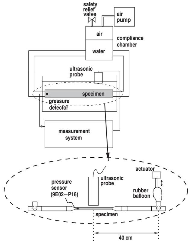
Fig. 3. Experimental system for basic experiments.
