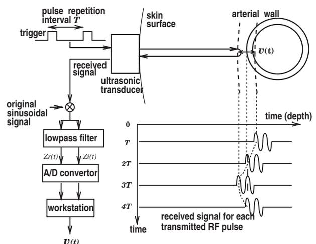
Fig. 1. Schematic diagram of the *phased tracking method*.
