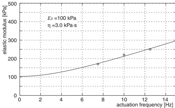
Fig. 13. Elastic moduli,  $|E_{\theta}^h(f_{ac})|$ , of a carotid artery measured at multiple frequencies (plot), and the estimated Voigt model (solid curve).
