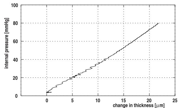
Fig. 9. Relationship between the change in wall thickness,  $\Delta h(t)$ , and the change in internal pressure,  $\Delta p(t)$ .
