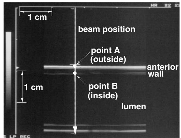
Fig. 5. B-mode image of a silicone rubber tube.
