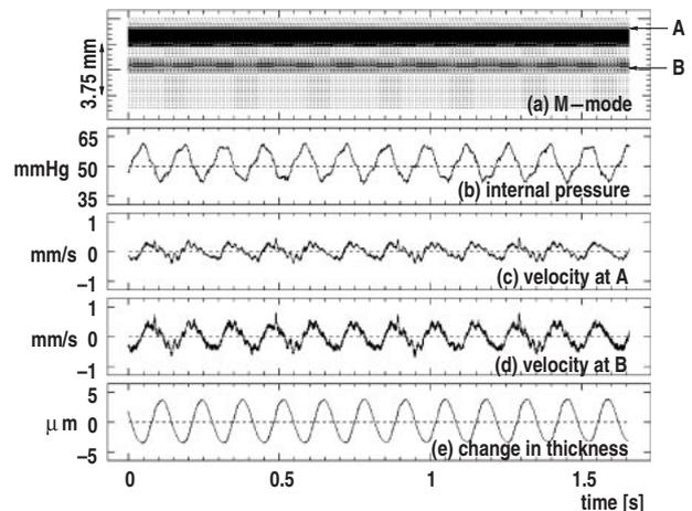
Fig. 6. (a) M-mode image of the silicone rubber tube. (b) Internal pressure. (c) Velocity,  $v_A(t)$ , of point A. (d) Velocity,  $v_B(t)$ , of point B. (e) Change in thickness,  $\Delta h(t)$ , of the anterior wall (actuation frequency of 7.5 Hz).
