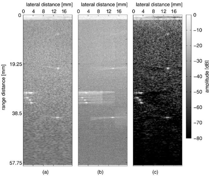
Fig. 9. B-mode images of string phantom obtained by (a) delay and sum beamforming (DAS), (b) amplitude and phase estimation beamforming (APES), and (c) modified amplitude and phase estimation beamforming (mAPES).
