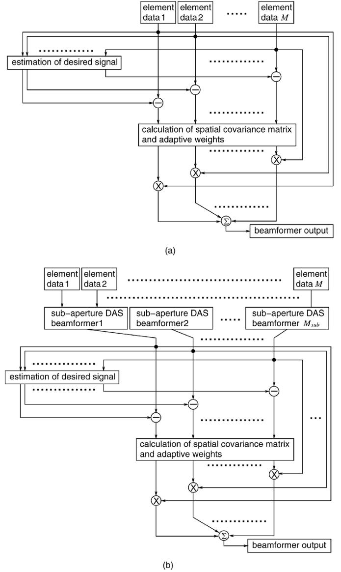
Fig. 2. Illustration of the proposed method with and without sub-aperture beamforming.
