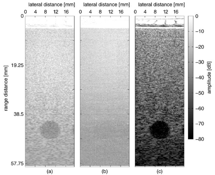
Fig. 11. B-mode images of cyst phantom obtained by (a) delay and sum beamforming (DAS), (b) amplitude and phase estimation beamforming (APES), and (c) modified amplitude and phase estimation beamforming (mAPES).
