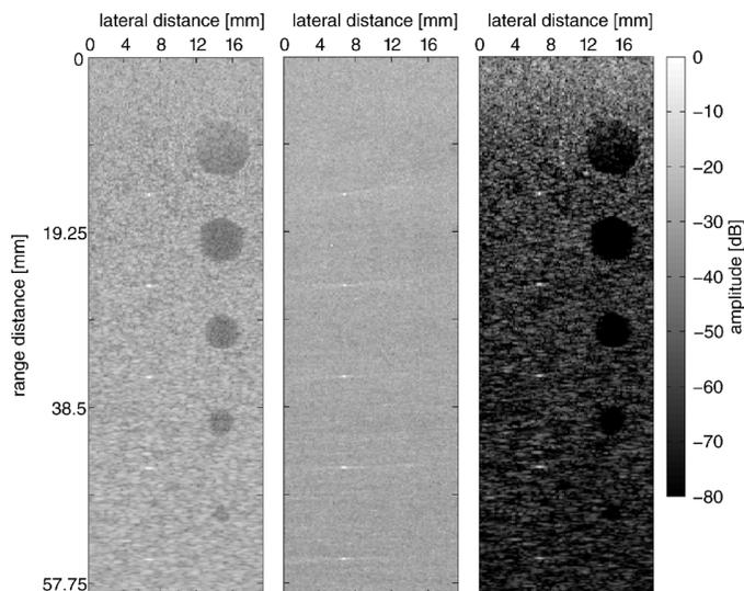
Fig. 4. B-mode images of simulated phantom obtained by (a) delay and sum beamforming (DAS), (b) amplitude and phase estimation beamforming (APES), and (c) modified amplitude and phase estimation beamforming (mAPES).
