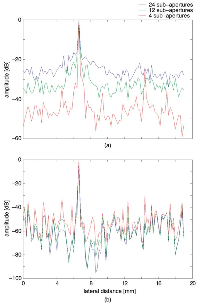
Fig. 7. Lateral amplitude profiles at a range distance of 15 mm in B-mode images shown in Fig. 6 obtained by (a) amplitude and phase estimation beamforming and (b) modified amplitude and phase estimation beamforming.
