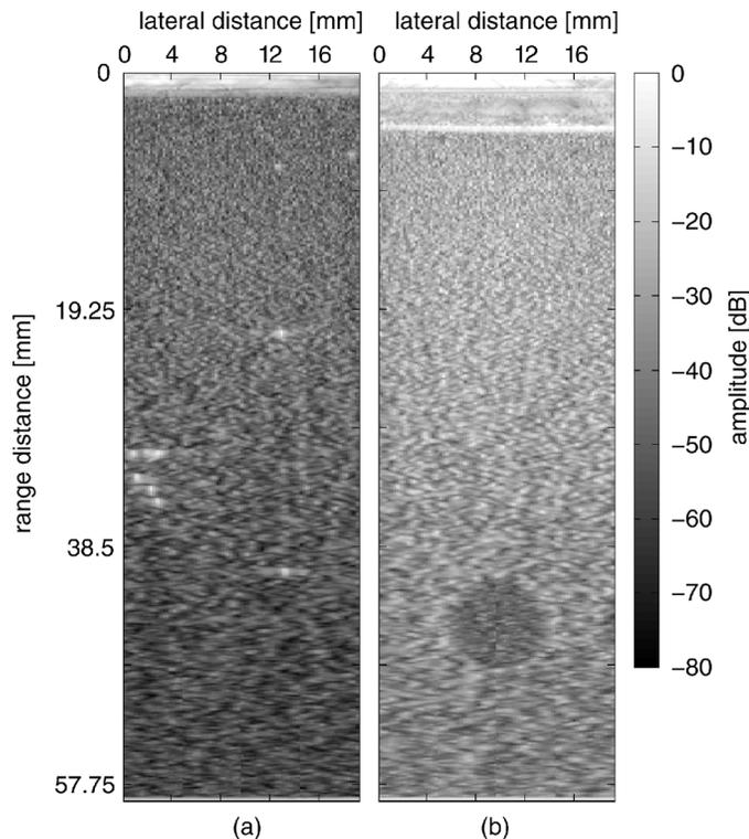
Fig. 16. B-mode images of (a) string and (b) cyst phantoms obtained by conventional APES beamforming with sub-array averaging (48 elements in each sub-array) and diagonal loading corresponding to  $0.05/L$  of the received power.
