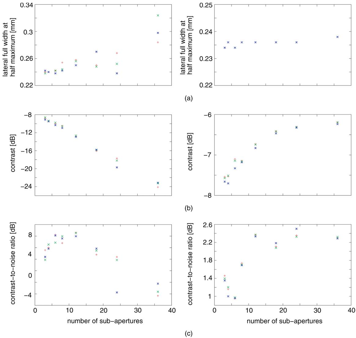
Fig. 8. Performance metrics obtained by (left) amplitude and phase estimation beamforming and (right) modified amplitude and phase estimation beamforming at different numbers of sub-apertures and signal-to-noise ratios (SNRs). (a) Lateral full widths at half maxima, (b) contrast, (c) contrast-to-noise ratios.
