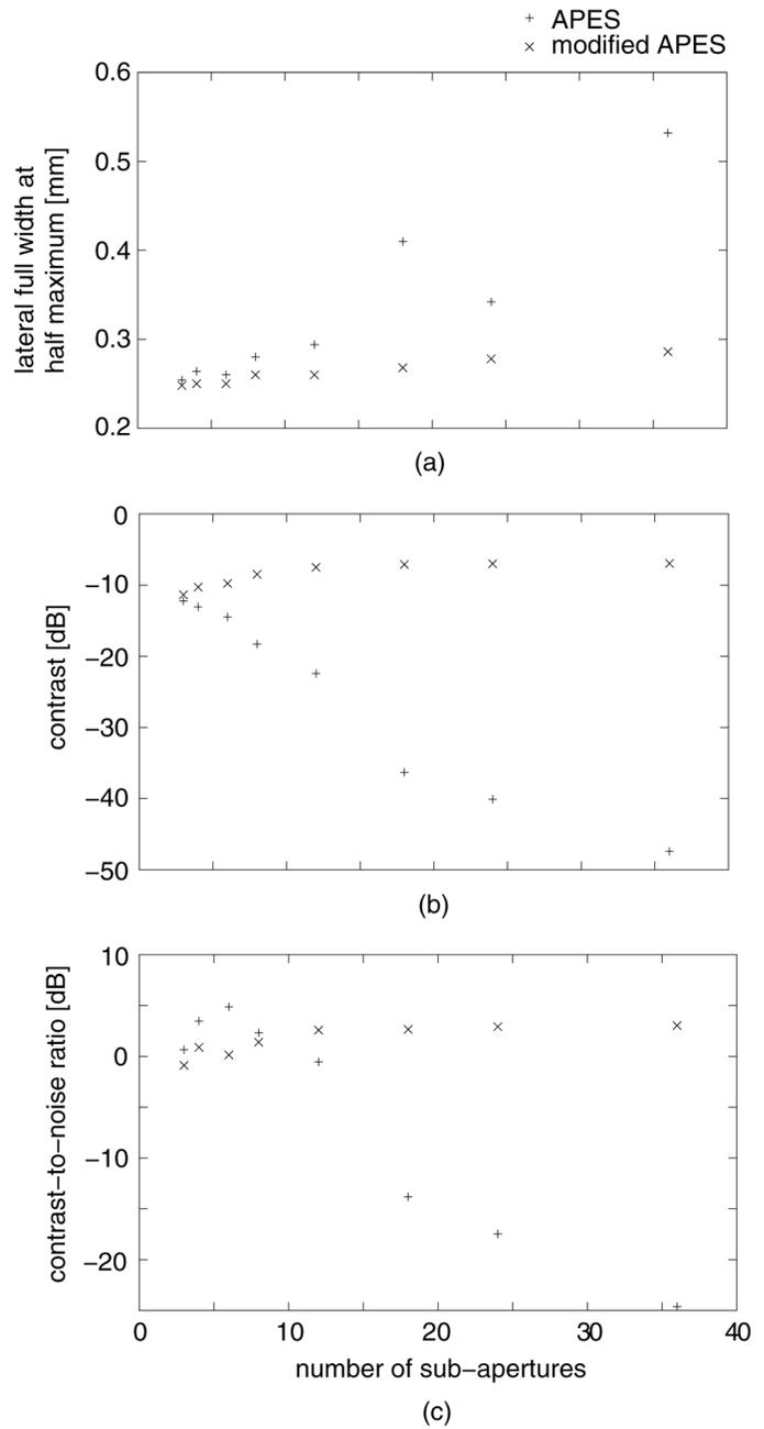
Fig. 15. Lateral full widths at half maxima (a), contrast (b), and contrast-to-noise ratios obtained by amplitude and phase estimation (APES) beamforming and modified APES with different numbers of sub-apertures.
