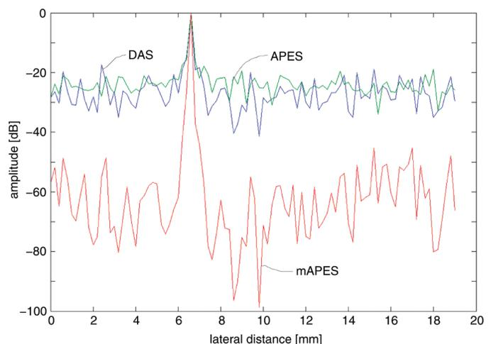
Fig. 5. Lateral amplitude profiles at a range distance of 15 mm in B-mode images shown in Fig. 4 obtained by delay and sum beamforming (DAS), amplitude and phase estimation beamforming (APES), and modified amplitude and phase estimation beamforming (mAPES).
