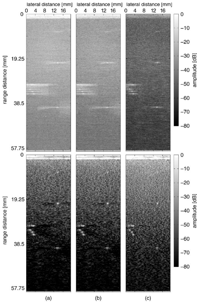
Fig. 12. B-mode images of string phantom obtained by (top) amplitude and phase estimation beamforming and (bottom) modified amplitude and phase estimation beamforming. (a) 24 sub-apertures, (b) 12 sub-apertures, (c) 4 sub-apertures.
