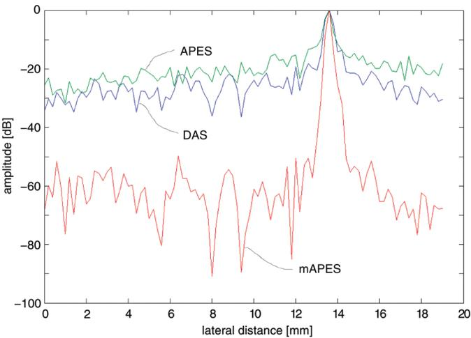
Fig. 10. Lateral amplitude profiles at a range distance of 21 mm obtained by delay and sum beamforming (DAS), amplitude and phase estimation beamforming (APES), and modified amplitude and phase estimation beamforming (mAPES).
