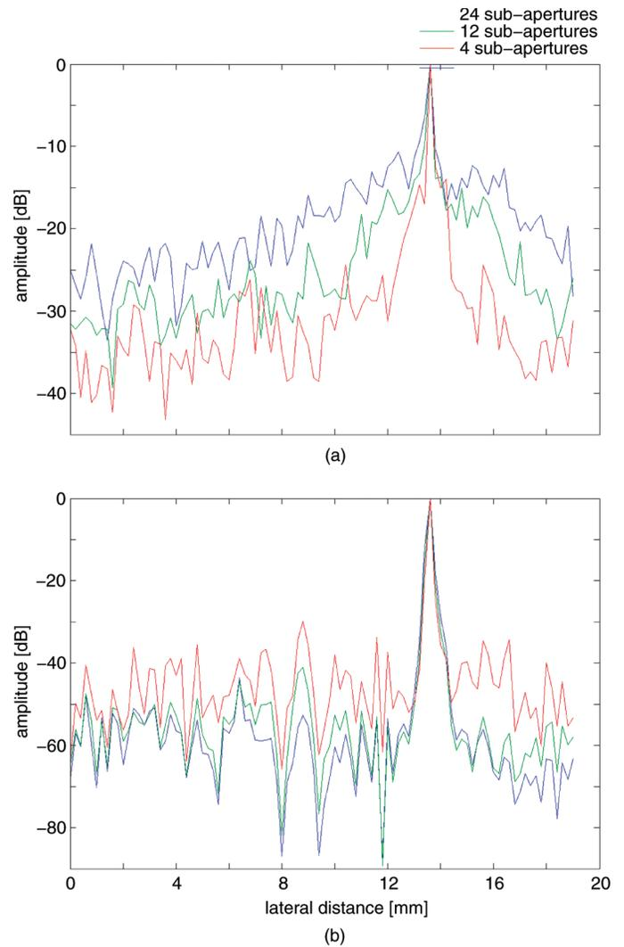
Fig. 13. Lateral amplitude profiles at a range distance of 21 mm obtained by (a) amplitude and phase estimation beamforming and (b) modified amplitude and phase estimation beamforming.
