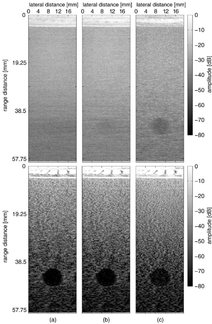
Fig. 14. B-mode images of cyst phantom obtained by (top) amplitude and phase estimation beamforming and (bottom) modified amplitude and phase estimation beamforming. (a) 24 sub-apertures, (b) 12 sub-apertures, (c) 4 sub-apertures.
