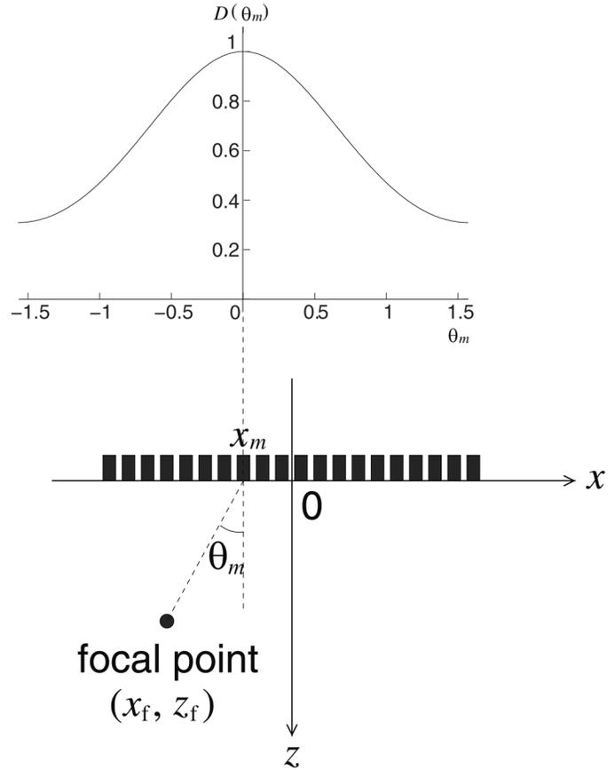
Fig. 1. Illustration of geometry. Directivity function  $D(\theta_m)$  was calculated by (11) at  $l = 150 \ \mu\text{m}$  and  $\lambda = 200 \ \mu\text{m}$ .
