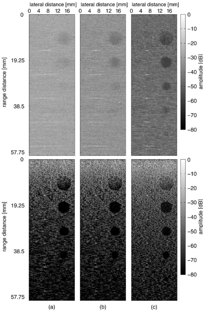
Fig. 6. B-mode images of simulated phantom obtained by (top) amplitude and phase estimation beamforming and (bottom) modified amplitude and phase estimation beamforming. (a) 24 sub-apertures, (b) 12 sub-apertures, (c) 4 sub-apertures.
