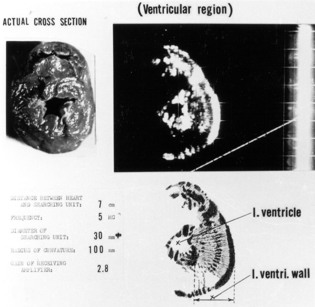
Fig. 1. High quality ultrasono-cardiotomogram (2-dimensional echocardiogram) of a canine heart at the left ventricular level obtained by using a concave disk transducer of 30 mm diameter, 100 mm radius of curvature, and 5-MHZ frequency. The heart just after excision was suspended at the focal area in the water bath. The echo pattern shows the three-layer structure.
