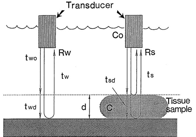
Fig. 3. Schematic representation of the principle measuring method for the thickness and speed of sound for a thin tissue specimen.
