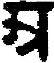
The thinned pattern is given by the black solid line and the original pattern is shown by the fuzzy part. Fig. 4 Result of the unmodified Holt algorithm for 'a'.
