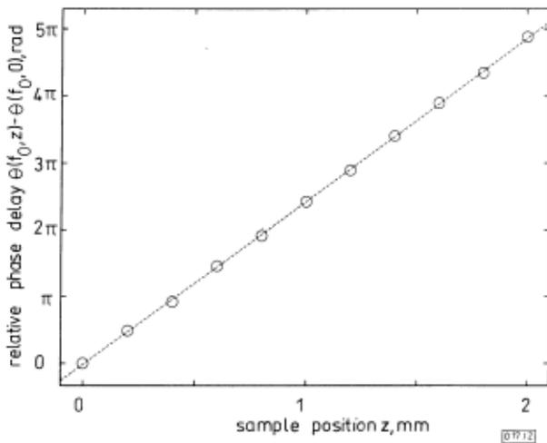
**Fig. 2** Phase change  $\theta$  in received signal measured for Bakelite sample
