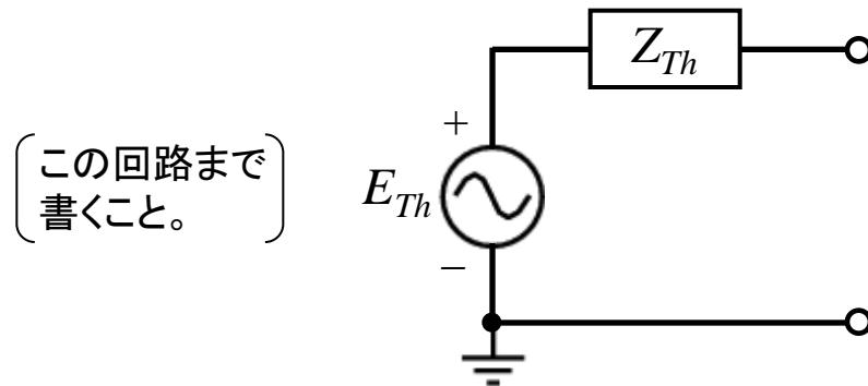
$$\left\{ \begin{array}{l} E_{Th} = \frac{X^2 - R^2}{X^2 + R^2} E_0 \\ Z_{Th} = \frac{2RX^2}{R^2 + X^2} \end{array} \right.$$
